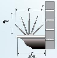
One row of Perma Spike Polycarbonate will cover 7" in width. Install Perma Spike Polycarbonate with at least 1/2" overhanging outer edge of Ledge, roof-line, window sill, etc.
