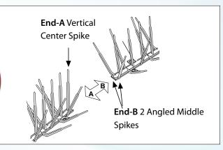
When Installing 2 or more lengths of spikes be sure to match End-A to End-B to prevent small openings where birds could land. *Apply End-A to End-B only!*
