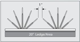
For areas greater than 7" in width - multiple rows of Perma Spike Polycarbonate may be used to ensure complete coverage. Do not leave more than a 1" gap between rows.
