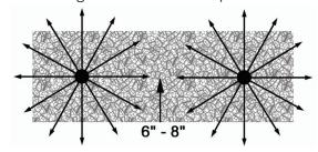
sure that they are installed 6-8" from arm tip-to-arm tip (not base-to-base).
