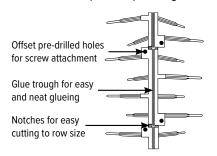
the screw holes for more effective adhesion. For a list of recommended adhesives, visit our website at birdbgone.com. One caulking tube of adhesive will adhere approximately 25 ft. of Bird Spike 2000®.
