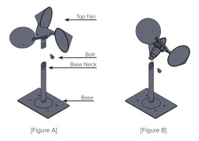
7. Use four (4) #10 screws to attach base to installation surface.
